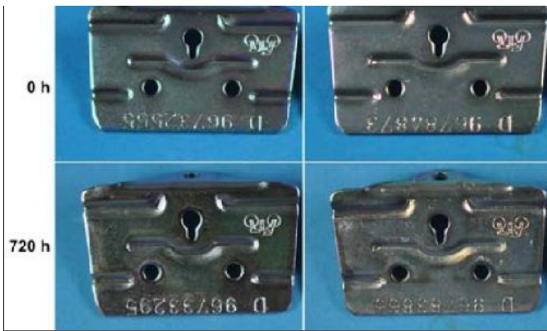
Figure 9 - Appearance of proprietary cobalt-free trivalent chromium passivate † on alkaline zinc after 720 hr of neutral salt spray (L) without heat treatment and (R) with heat treatment at 120°C for 24 hr.
