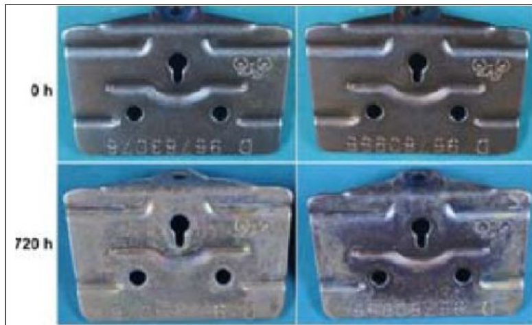
Figure 8 - Appearance of proprietary cobalt-free trivalent chromium passivate on zinc-nickel (12-15% Ni) after 720 hr of neutral salt spray (L) without heat treatment and (R) with heat treatment at 120°C for 24 hr.
