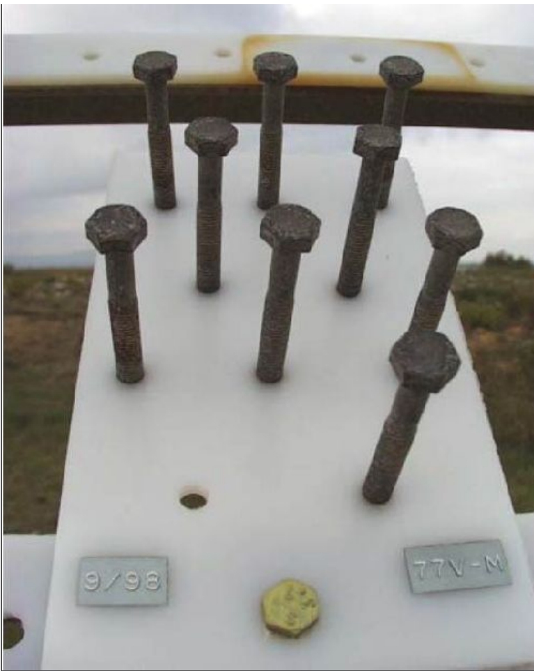
Figure 10 - Zn/Mn (>4% Mn) deposit after two years exposure to a seacoast atmosphere.
