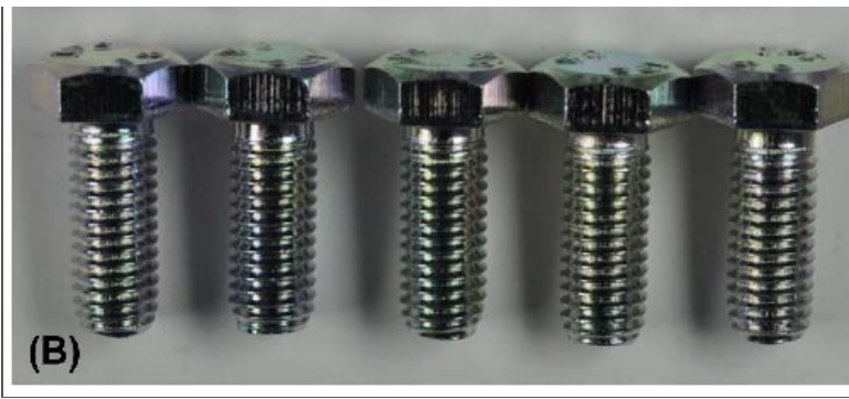
Figure 7 - Appearance of (A) cobalt-free and (B) cobalt-containing passivates on pure zinc after 72 hr of neutral salt spray.
